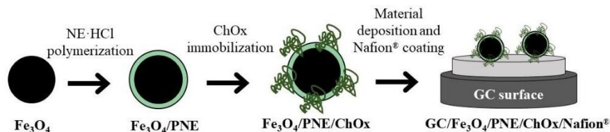
Fig. 1. Schematically presented stages of receiving the GC/ \text{Fe}_3\text{O}_4 /PNE/ChOx/Nafion ® biosensor
